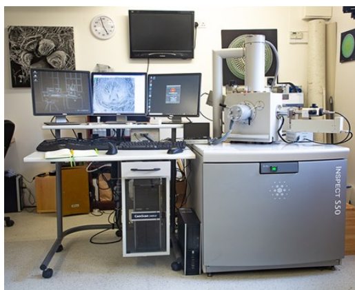
FEI Inspect S50 SEM with Deben Gen5 Back-Scattered Electron Detector fitted in the right hand port of the specimen chamber. The right-hand monitor displays the user interface for the detector. Also visible, beneath and to the right of that monitor, is the display for a Deben Chamberscope.
