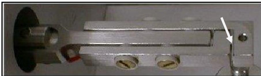
Older systems have tungsten plates which are a silver colour, the beam path is shown with an arrow above.
