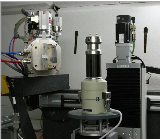
Figure 1: Deben CT5000-TEC mounted on University of Ghent's HECTOR micro-CT system.
