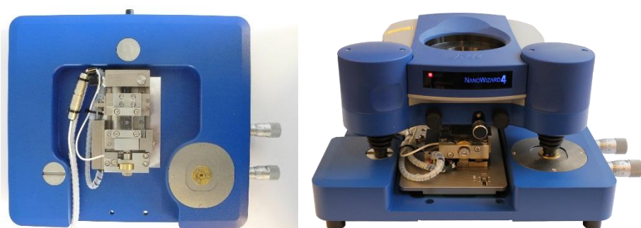
Deben Microtest 200N tensile and compression stage in use with the Nano Wizard AFM system.
