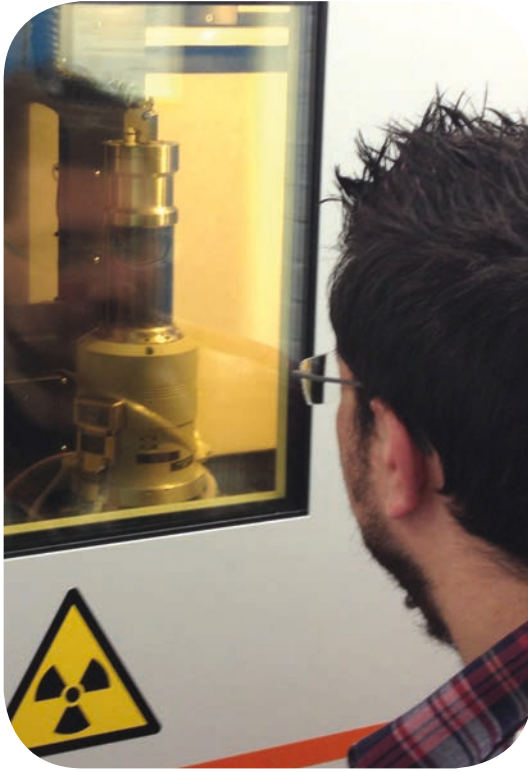
The Deben CT5000 tensile system mounted in a Nikon CT X-ray Inspection System at the University of Portsmouth.
