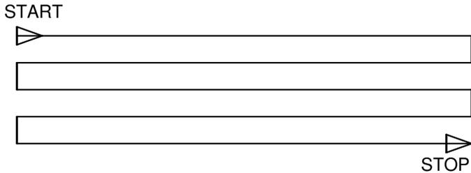
**RASTER** - scans horizontally across the sample in the positive direction only, then returns to start the next line at high speed:
