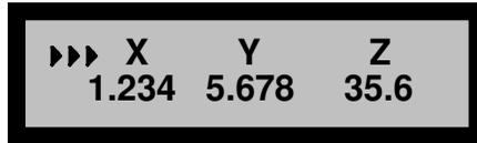
X/Y stage movement is controlled from the joystick and for Z, Tilt and Rotate movement, the labeled keys above the joystick are used. Z up will move the stage up ie. decrease working distance. Tilt up will increase the Tilt angle and Rotate up will rotate the stage in a clockwise direction (on the visual monitor).
