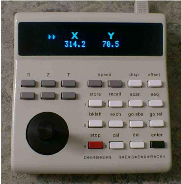
The co-ordinate display is angled at 15° to ensure that it may be viewed at a distance. A speed proportional analogue joystick is used for accurate movement of X/Y axes and independent keys are provided for control of Z (working distance), Tilt and Rotate of the specimen sample.
